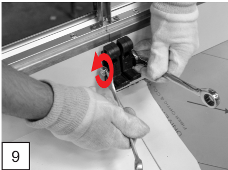
9 Connecting devices with each other via delivered fasteners
